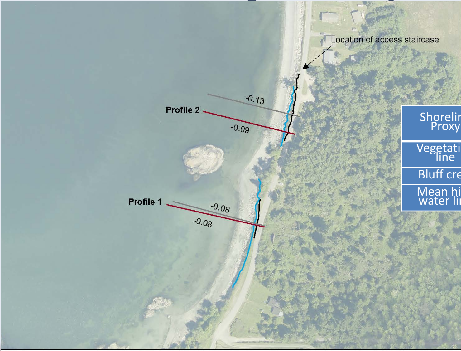
Figure 11. Bluff crest erosion along the southern stretch of Outer Bay beach from 1977–2016. Erosion rates are given in FT/YR. Mackaye Harbor Road Relocation Feasibility Study
