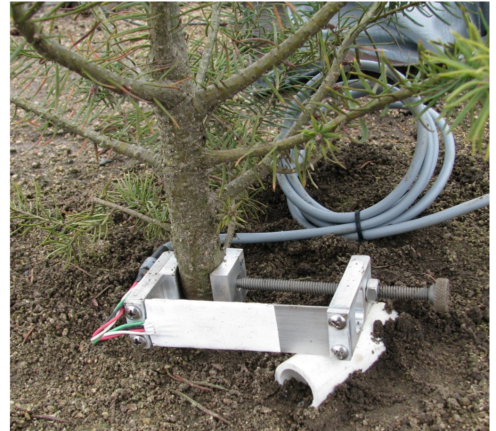
Electronic dendrometers measure tree size every 30 min
